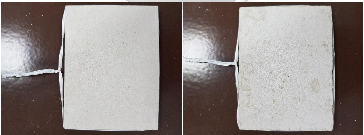
Figure 3: Photos (both sides) of test specimen - replicate 3 at the end of testing (Rating =10).
